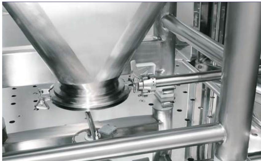
Automatic opening of the lower bin valve
