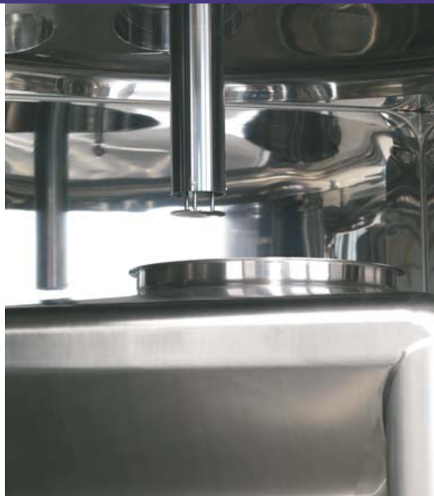
Telescopic tube for internal BIN drying
