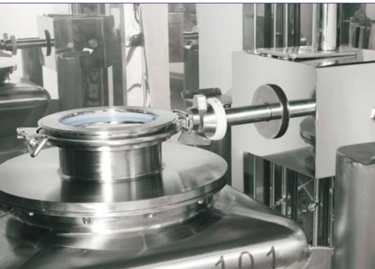
Automatic opening of the upper bin valve.
