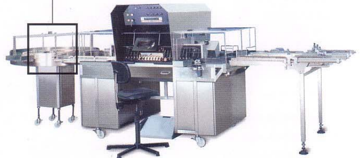
VISOMAT IV-2 with upstream turntable DT 1200 for inspection of lyophilised vials.
