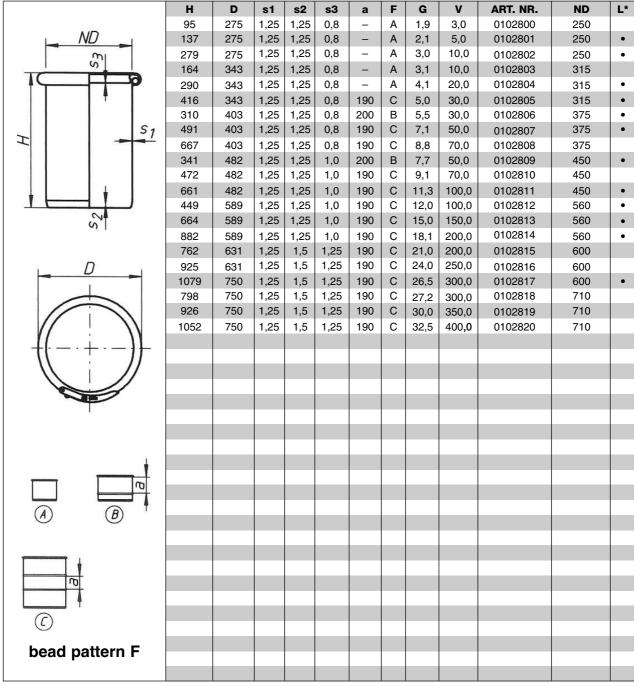
H = drum height, D = outside diameter, s1 = body sheet thickness, s2 = base sheet thickness, s3 = lid sheet thickness, F = bead pattern, G = weight in kg, V = volume in litres, ND = nominal diameter, L ● = to be preferred
