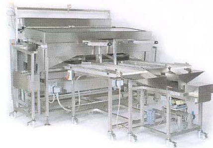
SORTOMAT 20 with subsequent inspection and weighing.
