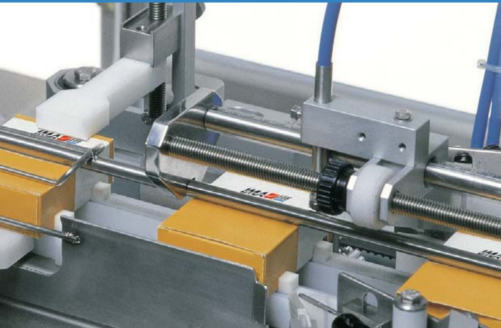
A double eccentric continuous motion device folds the labels as the cartons pass
