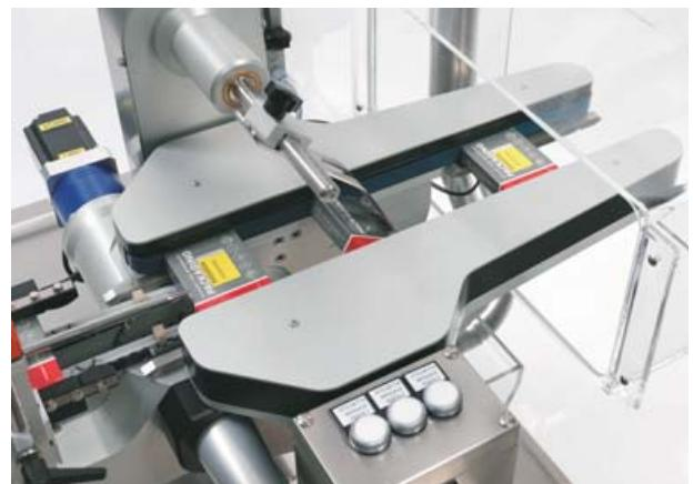
The rejection unit is also designed according to the latest GMP's regulations, allowing maximum visibility of the whole labelling process. It consists of a positive logic pneumatic flap to carry out the rejection of non conforming cartons with missing label and/or faulty printed data into a box positioned inside machine basement on operator's side.
