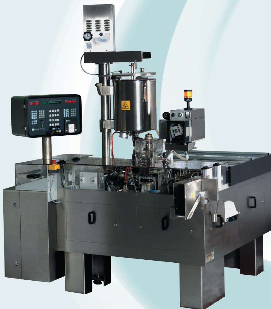
Automatic machine for the production of suppositories in aluminium or plastic formed cavities
