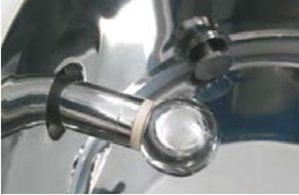
TwinValve cleaning spray head in extracted position, vacuum open
