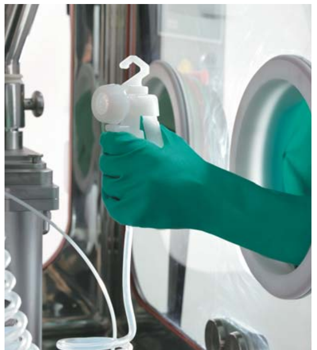
Spray gun inside the process area
