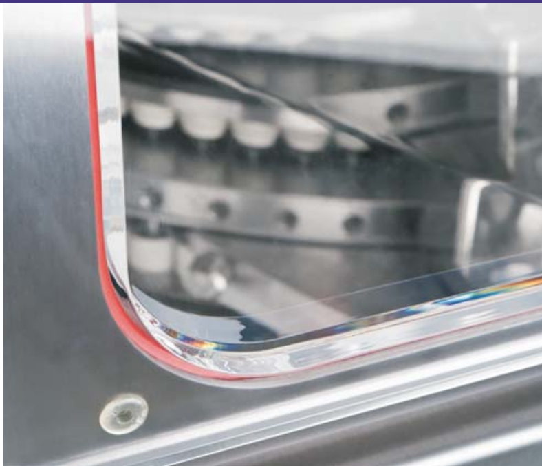
Machine door: deflated seal
