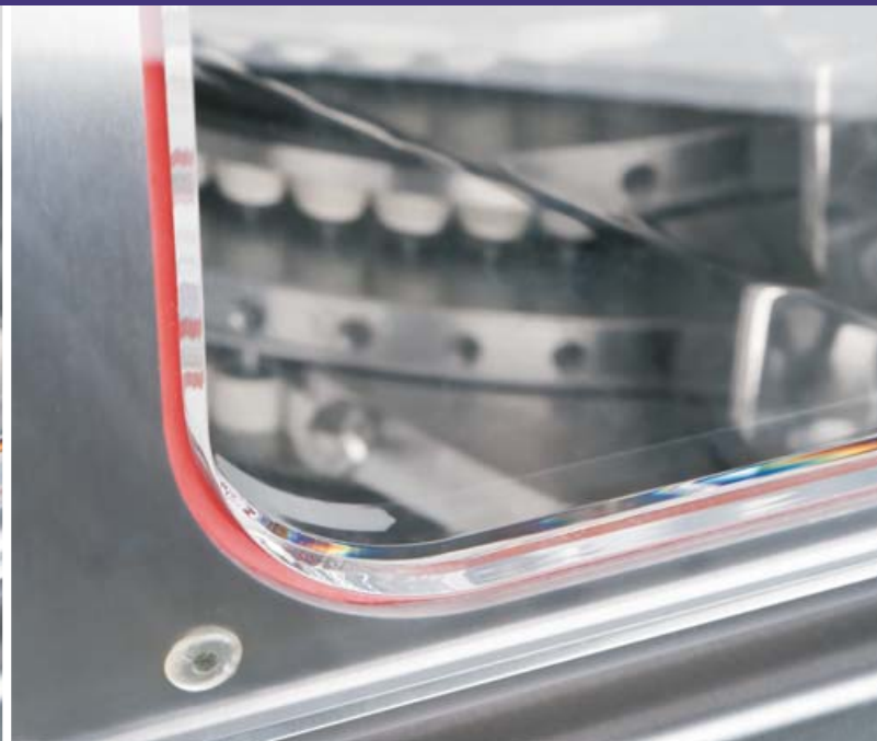
Machine door: inflated seal
