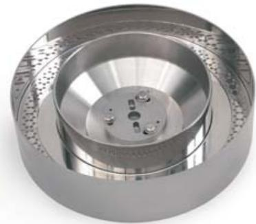
In addition to the rotary bowl fitted on standard machines, the IMA patented vacuum bowl can be supplied for powder pre-compacting in case very fine powders have to be dosed.
