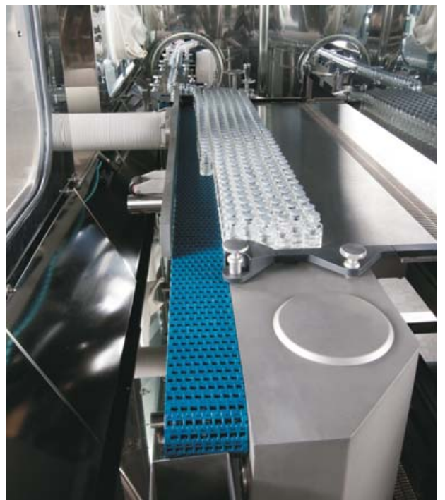
Fixed system integrated with a complete aseptic filling line under isolator.
