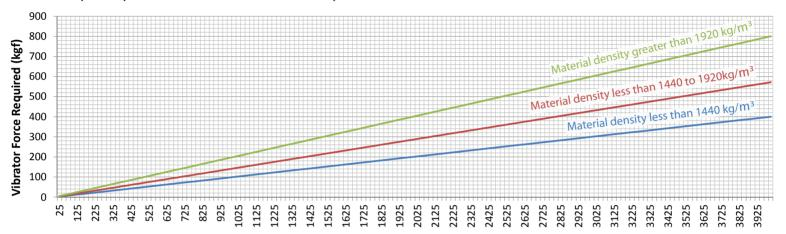
Weight of Material in Conical or Taper Section (kgs)
