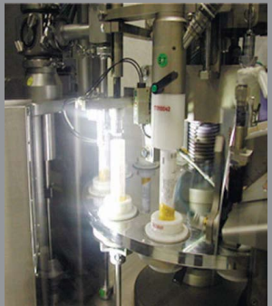
ROTATING TUBES INSPECTED BY TLC
