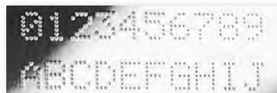
Example of standard typeface 5 x 7 point matrix with 5 mm font size.
