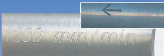
CrNi Steel, marking onto the radius w/o height correction
