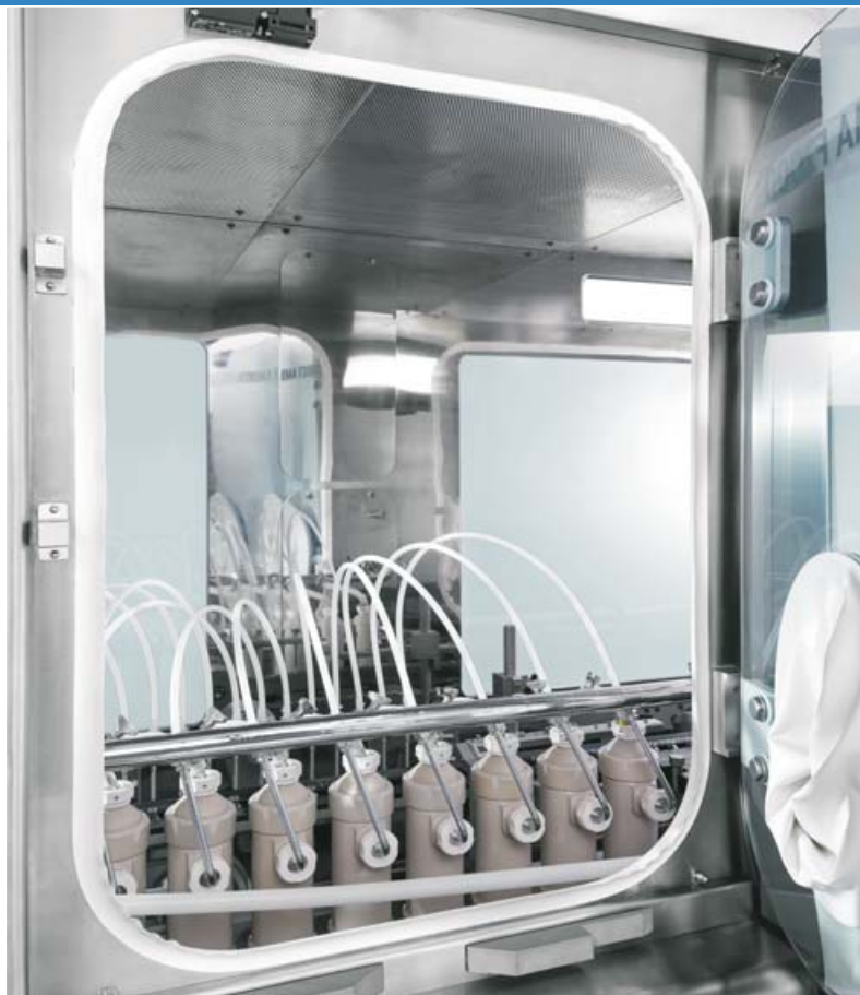
Gaskets and details of filling area
