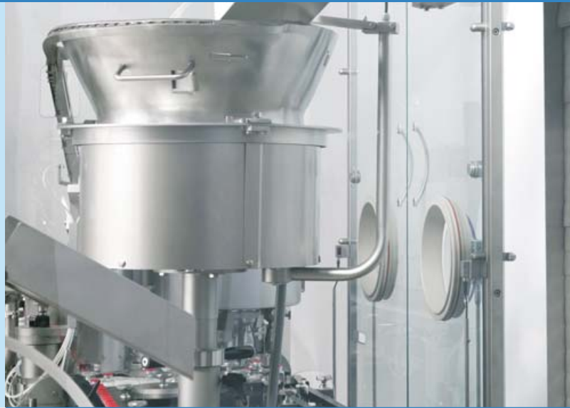
SEPARATE CONTAINMENT AREA FOR ALU CAP FEEDING
